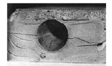
This mold shows obvious signs of not having been packed fully enough. Separate layers of rubber are easily visible, as are air bubbles.
